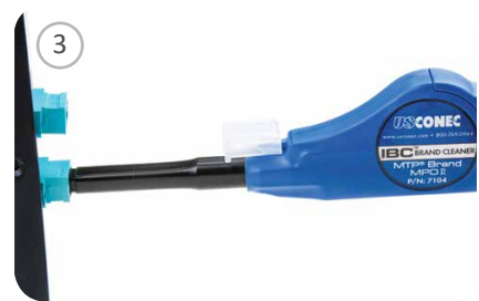
3 Follow standard cleaning procedure for connector type and cleaner used. A second push will provide a dry clean
