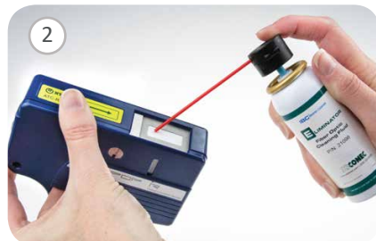
2 Spray a very small amount of cleaning solvent on one end of the cleaning cloth. Do not soak the cloth. Excessive cleaning solvent will require additional dry cleans
