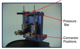
**Step 4:** Lift connector positions upward using the pressure bar. Slide upper pin beneath bar to hold.
