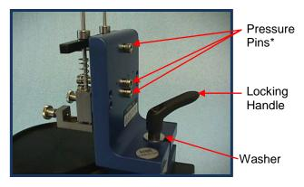
**Step 3**: Engage workholder with base post. Make sure the washer sits between locking handle and workholder. Align workholder square with polisher and lock.
