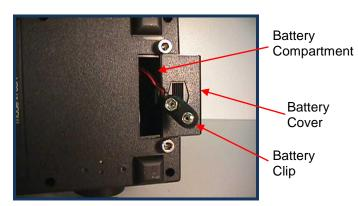
**Step 1:** Power SpecPro<sup>™</sup> with either its AC adapter or a 9 volt battery. WARNING: USE ONLY THE AC ADAPTER SUPPLIED BY KRELL.
