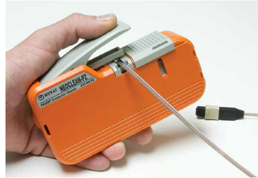
Cleaning PRIZM® LightTurn® connector
